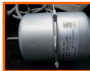
FAN MOTOR ( CONDENSER SIDE) YDK95-50-6DL (A015-12L-203D) 000466 2A01 220V ~ / 60Hz / 0.5A / 50W / 5uf / 450V
