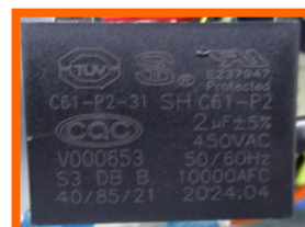
FM CAPACITOR 1 st CBB61 / 5uf / +/-5% / 450VAC / 50-60Hz 2 nd 2uf / +/- 5% / 450VAC / 50-60Hz CP1-P2-31 / SH C61-P2
