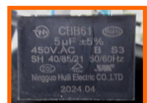
FM CAPACITOR 1 st CBB61 / 5uf / +/-5% / 450VAC / 50-60Hz 2 nd 2uf / +/- 5% / 450VAC / 50-60Hz CP1-P2-31 / SH C61-P2
